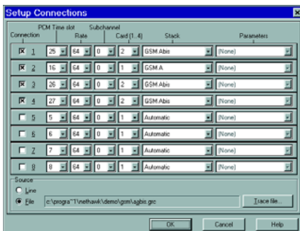
Selection and definition of timeslots to be monitored on GSM analyzer
